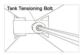
Note: Do not over tighten Tank Bolts.
